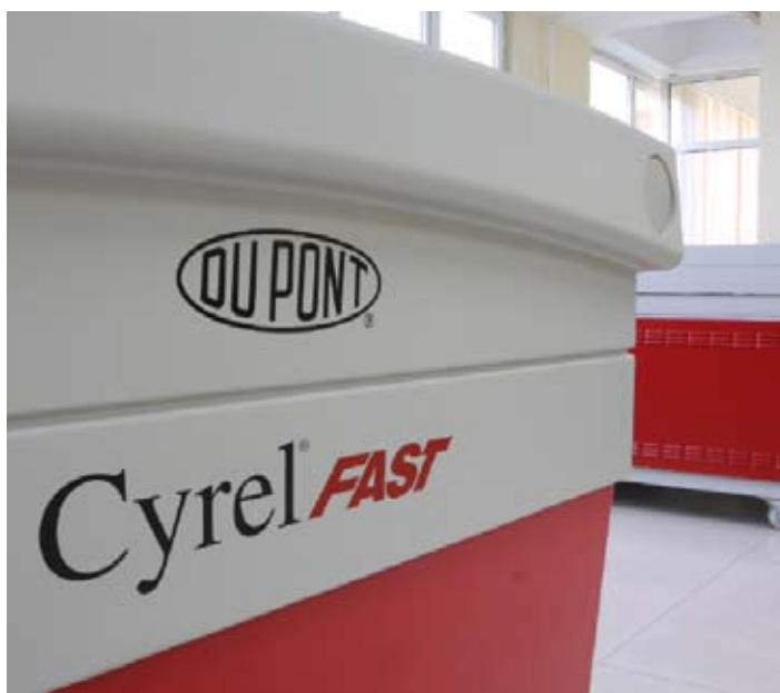
DuPont™ Cyrel® FAST 1000 TD - thermal plate-making process without solvents
