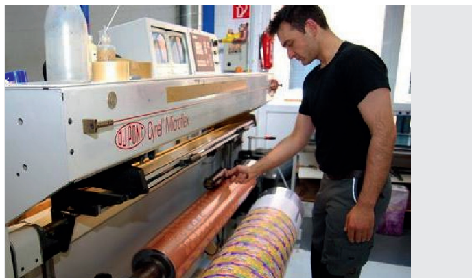
Final "test run" at manufacturer: Individual printing plates were combined to form complete print forms on this round assembly machine and proofing press
