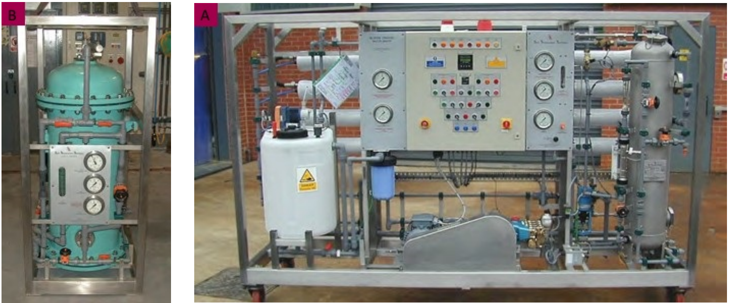
Figure 1: Images of Rothera plant (A. Sand filter and B. RO unit), courtesy of Salt Separation Services, UK.
