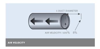
**Remember:** The hood should be as close to the source as is practical. Tests have shown that the air velocity diminishes rapidly as the distance from the hood opening is increased (see sketch before).
