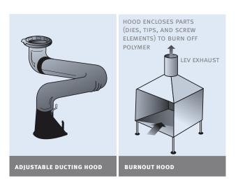
2. The hood should be shaped to enclose the source as far as is practical yet still allow access to the equipment for normal operation. The hood should be removable or connected to an adjustable duct that can be moved aside from extrusion or moulding equipment for maintenance or trouble-shooting. Adjustable ducting of this type is commercially available. Care should be taken to avoid kinking or excessive lengths of flexible tubing.
