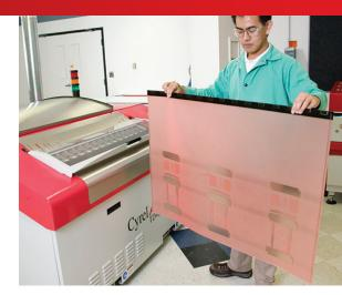
DuPont™ Cyrel® DFR is the high durometer plate for the DuPont thermal platemaking process, designed to meet the needs of high quality flexo with finest halftone, linework and solids.
